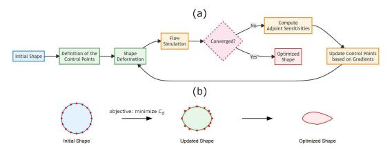
A discrete adjoint framework has been shown to facilitate efficient aerodynamic optimization by leveraging adaptive polynomial chaos expansion to mitigate uncertainties in flow conditions, improving design robustness significantly (Zhang et al.,
