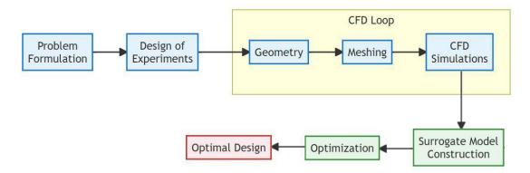
SBO has found widespread applications in engineering that require complex simulations and high-dimensional optimization, especially in aerospace and turbomachinery design. Its effectiveness has been demonstrated in diverse disciplines, including aerodynamics, structures, and propulsion.
